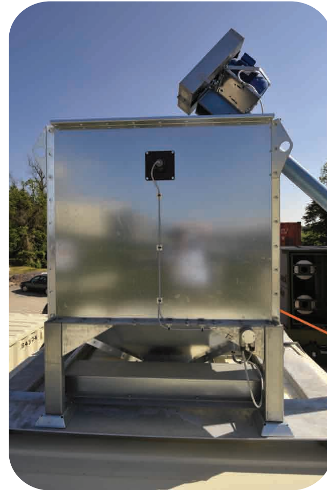
↑ Feed hopper skid mounted onto expelling container for quick removal by forklift/telehandler.
