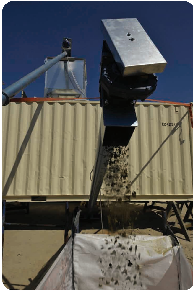
↑ Cake auger collects from chute underneath container and delivers to bulk bag
