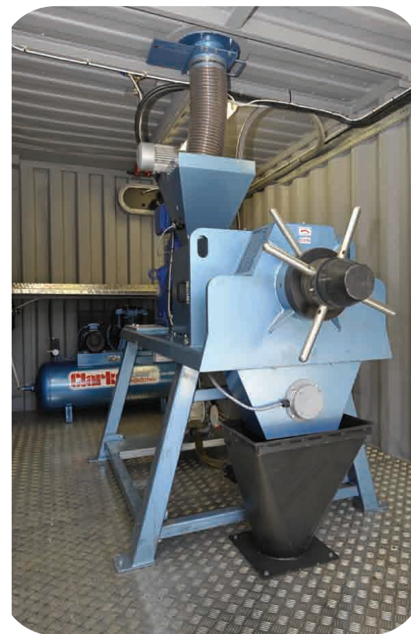
↑ Hopper feed gate is open and seed flows down into the oil expeller below.
