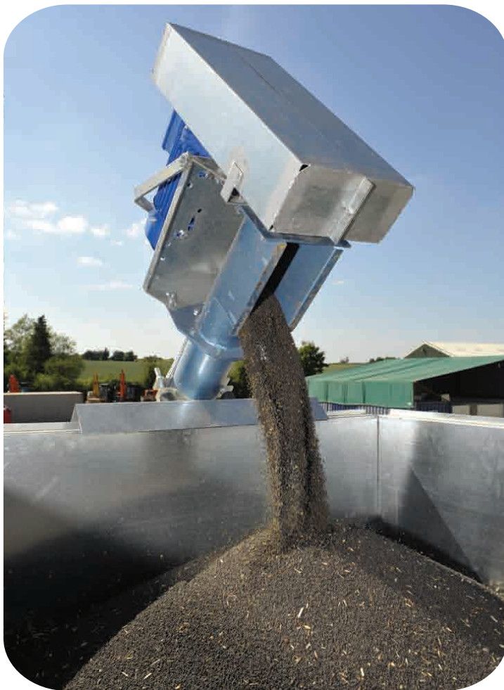
↑ Auger delivers OSR (oilseed rape) to overhead hopper.
