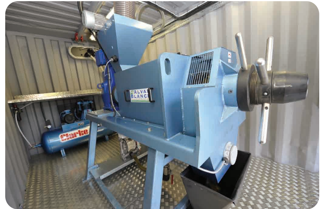
↑ Cake exits the press into the collection hopper below
